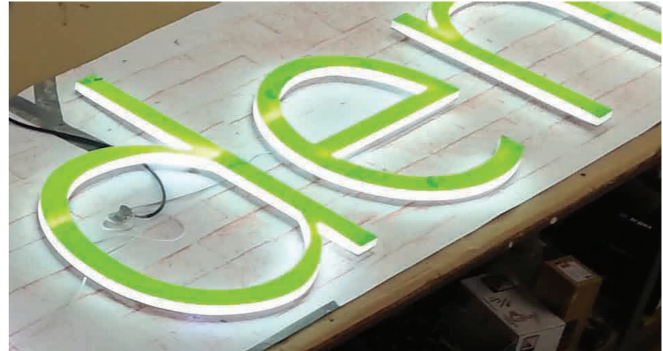
Built up acrylic with face and return illumination (80mm deep)
